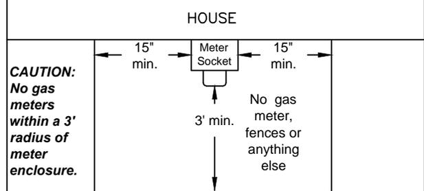
For residential service, the meter is to be located on the outside of the building on the side of the residence within three feet of the front wall and outside of the fences on the side most economical to reach the company's facilities.
