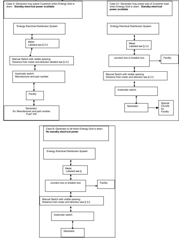
Note: A one line diagram submitted to the Company could be like the ones above with equipment specific information included
